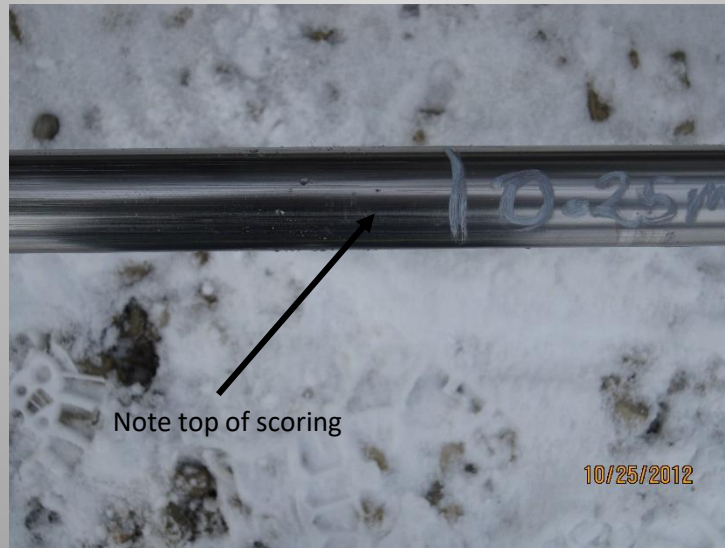
Measurement indicating tubing hanger position on polished rod and the top of the scoring.
