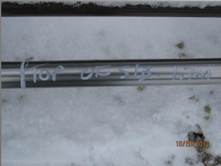
Measurement from top of stuffing box to tubing hanger at the bottom of the pumpjack stroke.
