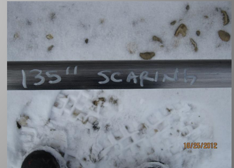
Measurement indicating total length of scoring on polished rod.
